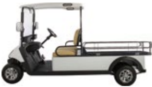
· Shuttle A/B铁货箱 铁货箱尺寸:1735*1160*350 mm
